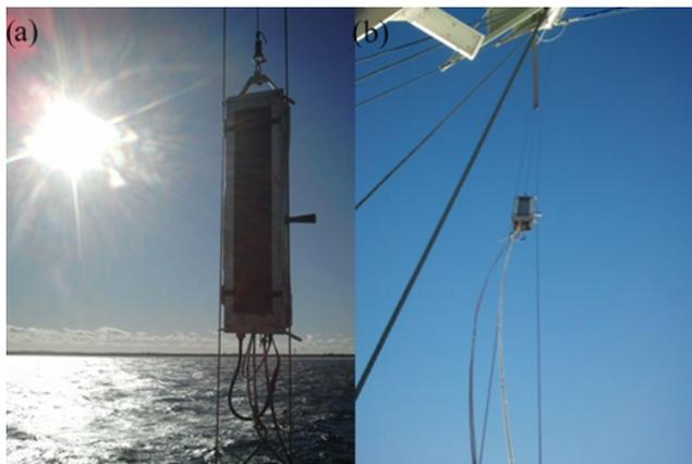
**Figure B1.** The classical aerosol spectrometer (left) and the method of the device moving between altitude levels during gradient measurements (right).
