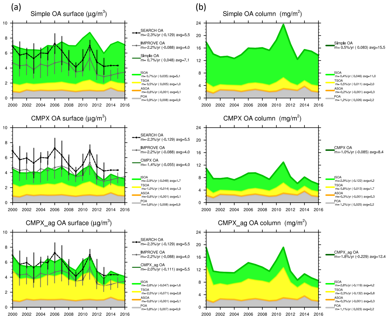
Figure S1. Summertime (a) surface and (b) column concentrations of OA in the SEUS. Color shades represent OA components from each scheme. In attached text, “m” represents 2000-2016 relative trend with units of %/year; numbers in parenthesis in (a) and (b) represent trends with units of \mu\text{g}/\text{m}^3/\text{year} or \text{mg}/\text{m}^2/\text{year} ; “avg” represents the 17-year average with units of \mu\text{g}/\text{m}^3 in (a) and \text{mg}/\text{m}^2 in (b).
