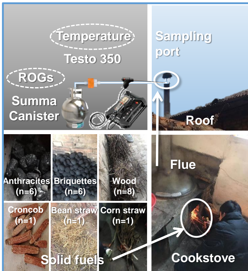
Figure S1. Sampling diagram relates to six solid fuels types, household stoves, sampling port and equipment. The letter n refers to the number of different samples.
