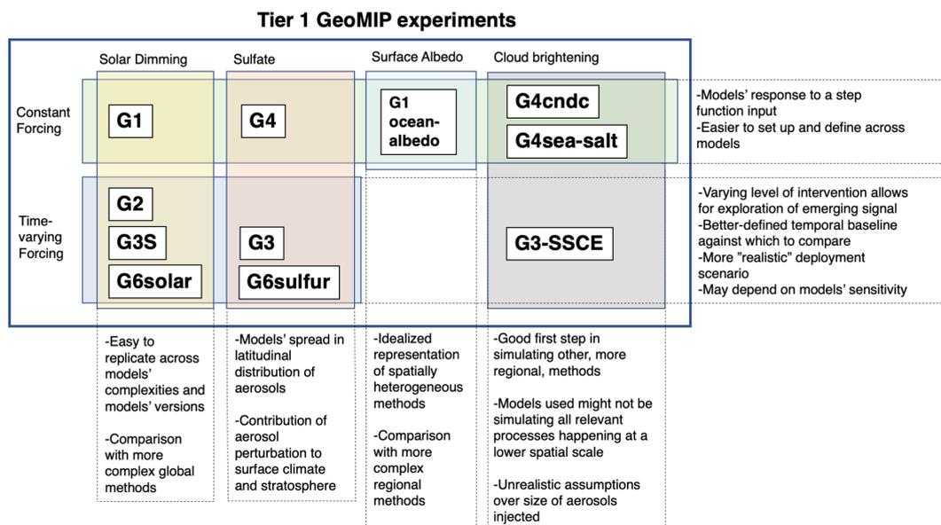
**Figure 1.** Schematic summary of all Tier-1 GeoMIP experiments across different iterations (Kravitz et al., 2011, 2013, 2015). In rows, experiments are categorized based on how the geoengineering forcing is applied: constant or time-varying. In columns, experiments are categorized based on the method of applied forcing. Reference scenarios for each experiment are listed in Table 1.
