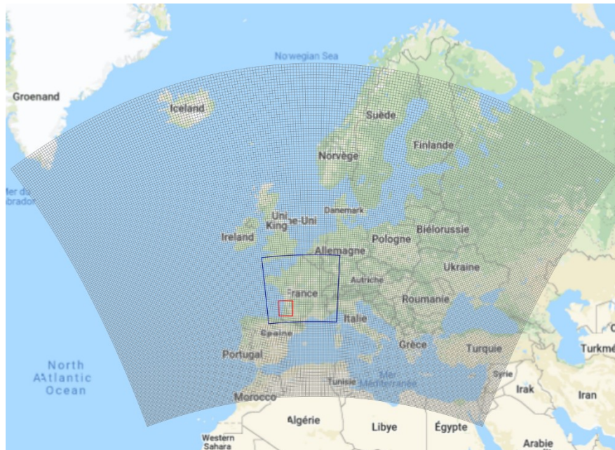
Figure S1: Domains used in the study: 1: European coarse domain (25kmx25km horizontal resolution), 2: French intermediate domain (5kmx5km horizontal resolution) and 3: high-resolution domain (1kmx1km horizontal resolution). © OpenStreetMap contributors 2022. Distributed under the Open Data Commons Open Database License (ODbL) v1.0.
