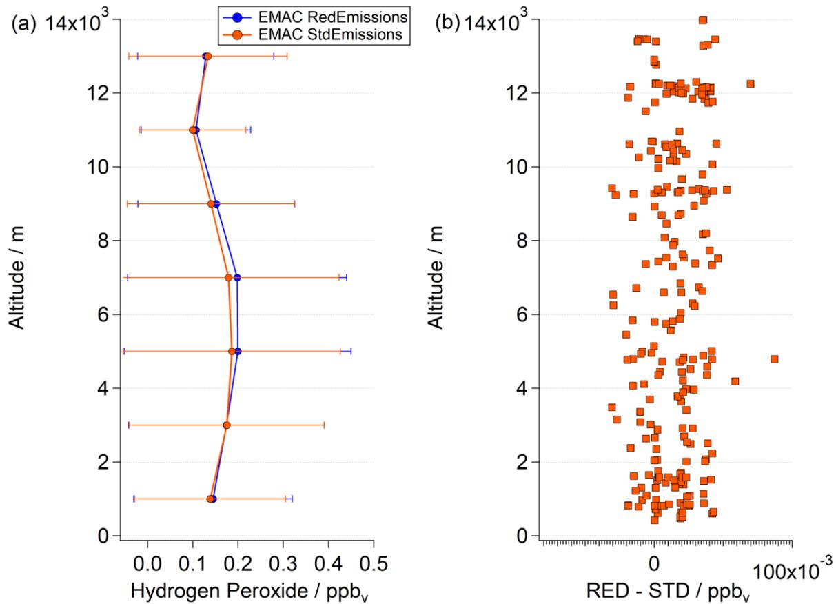
45 **Figure S4: Vertical profiles of hydrogen peroxide with (blue) and without (orange) the CORONA lockdown emission reductions (a) and absolute difference of the modelled mixing ratios (b). In order to examine the impact of the reduced emissions on the budget of H<sub>2</sub>O<sub>2</sub>, the entirety of both datasets provided by EMAC was used. Please note that the data was not filtered analogously to the procedure described in Sect 3.1.**
