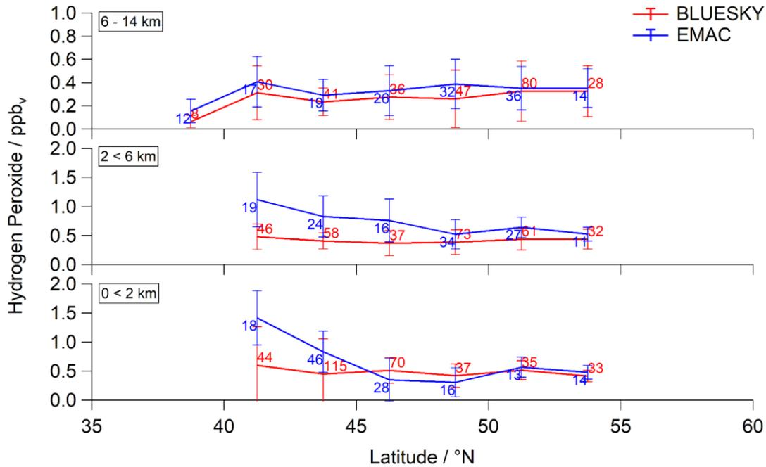
35 **Figure S3: Latitudinal distribution of hydrogen peroxide in comparison to model EMAC (red: BLUESKY; blue: EMAC). The data was subdivided into three atmospheric layers, upper troposphere, middle troposphere and boundary layer (from top to bottom) with mean values binned for 2.5° of latitude for each tropospheric layer. The corresponding numbers indicate the total amount of data points per bin.**
