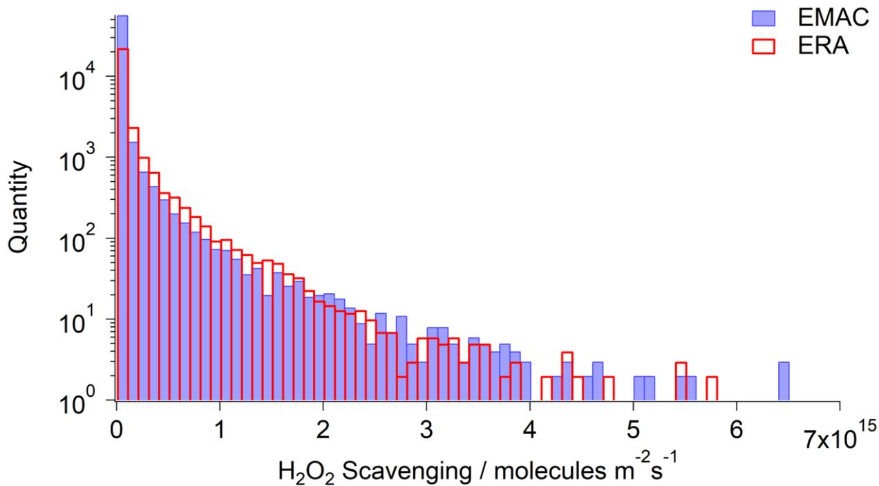
85 **Figure S8: Histogram of the hydrogen peroxide scavenging modelled by EMAC (blue) and the predicted scavenging by ERA5 (red). The scavenging data of ERA5 were obtained by extrapolation based on linear regression between scavenging and precipitation by EMAC.**
