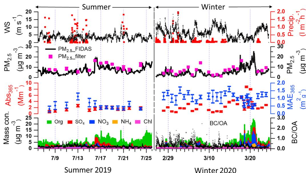
**Figure 1.** Time series of wind speed, precipitation, PM<sub>2.5</sub> mass concentrations from FIDAS optical particle sizer and gravimetric analysis of filter samples, optical properties of methanol-soluble aerosol particle compounds (Aqualog), concentrations of non-refractory aerosol particle compounds (AMS), and ratios of BC/OA in summer 2019 and the following winter.
