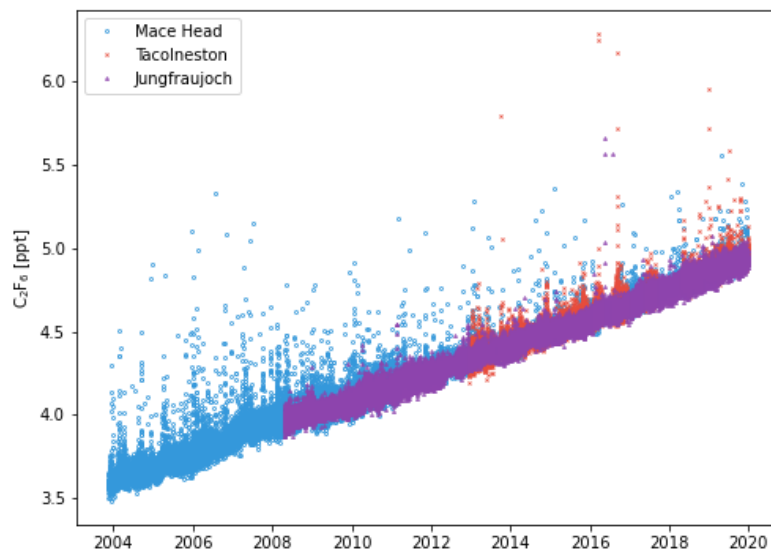
Figure S2. European observations of C_2F_6 measured at Mace Head (blue circles), Jungfraujoch (purple triangles) and Tacolneston (red crosses) from December 2003 – December 2019 inclusive.
