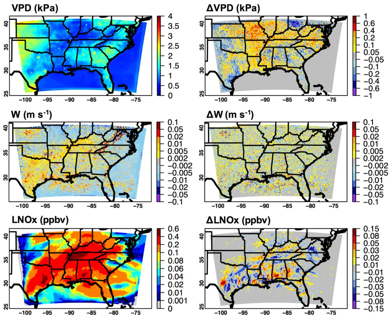
Figure S7. Period-mean (16-28 August 2016) WRF-Chem daytime (upper) surface vapor pressure deficit, VPD; (middle) vertical wind speed  $W$  averaged from surface level to  $\sim 200$  hPa, with noises near the domain boundaries screened; and (lower) lightning  $\text{NO}_x$  ( $\text{LNO}_x$ ) tracer results at  $\sim 400$  hPa. The left panels present the base case results, and the SMAP DA impacts on these model fields are shown in the right panels.
