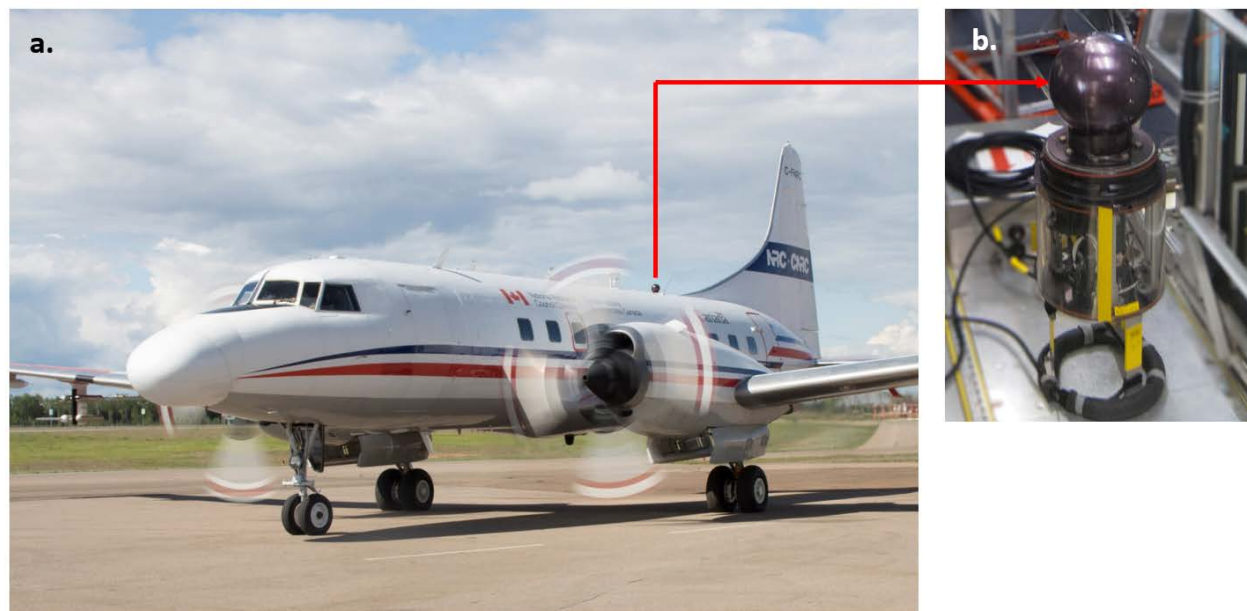
Figure S1: 4STAR at Fort McMurray installed on the Convair-580 aircraft; b. 4STAR head and its optical cables sitting inside the aircraft during routine maintenance
