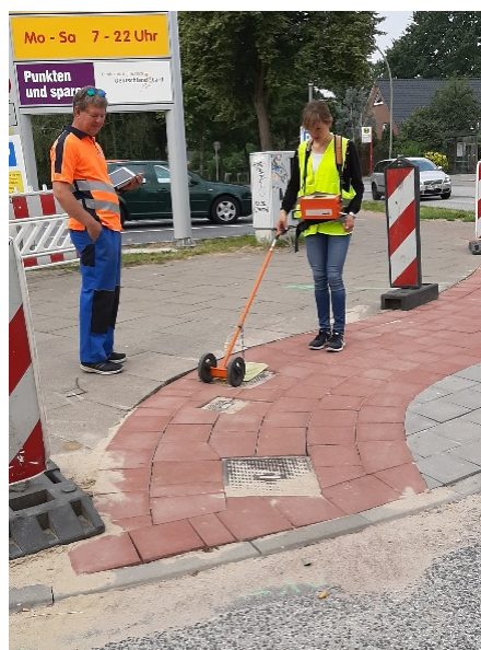
Figure S18: Leak detection operation by GasNetz Hamburg
