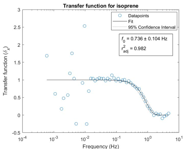
**Fig. S2.** Transfer function of the VOC eddy covariance system calculated for isoprene. Values calculated experimentally (datapoints) and fit to the one parameter sigma function (solid line) with 95% confidence interval (dotted lines).
