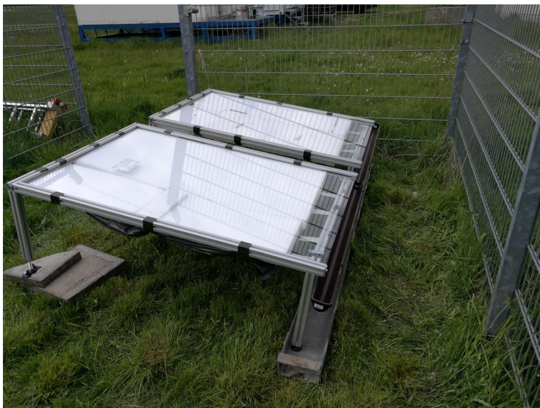
Fig. S2. The dew collector system: The glass sampler surface is 1.0 \times 1.5 \text{ m}^2 , and about 40 cm above ground at the lowest point.
