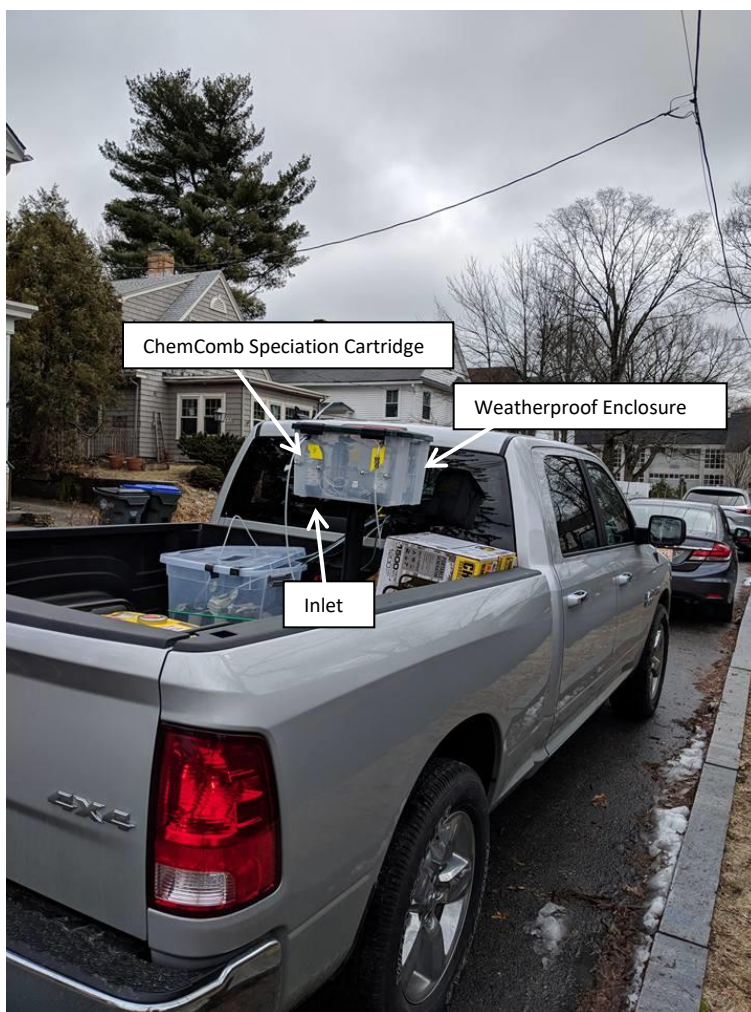
Figure S3: Image of the mobile lab for on-road collections of \text{NH}_3 from fresh vehicle traffic plumes in the northeastern US. The collection of \text{NH}_3 was conducted using a ChemComb Speciation Cartridge, which was held in a weatherproof enclosure, and the sampling inlet was directly exposed to ambient air to limit the inlet loss of \text{NH}_3 .
