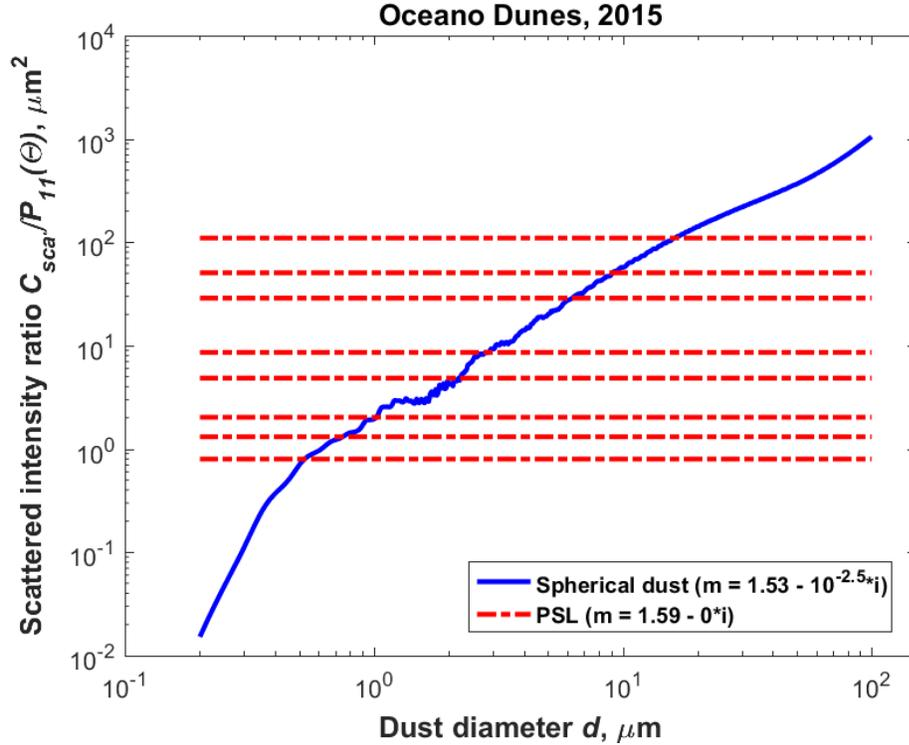
Figure S4: The ratio of scattered light intensity to incident intensity,  $C_{sca} \int P_{11}(\theta)$ , as a function of particle diameter using Lorenz-Mie theory. The figure includes the ratios for each of the eight polystyrene latex spheres (PSLs) boundary diameter sizes (thus seven size bins) (red dash-dot lines) (Table 1, column 1) and the ratios for dust particles with various geometric diameters (blue line).
