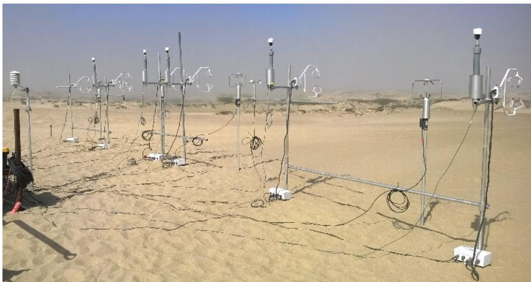
10 Figure S2: The experimental configuration of the five optical particle counters (OPCs) (with Series ID 9284, 9290, 9281, 9278 and 9287, respectively) at the same height (1.95 meters) above the surface and in a line perpendicular to the wind during June 5<sup>th</sup>, 6<sup>th</sup> and 7<sup>th</sup>, 2015, collecting aerosol number concentrations for OPC intercalibration.
