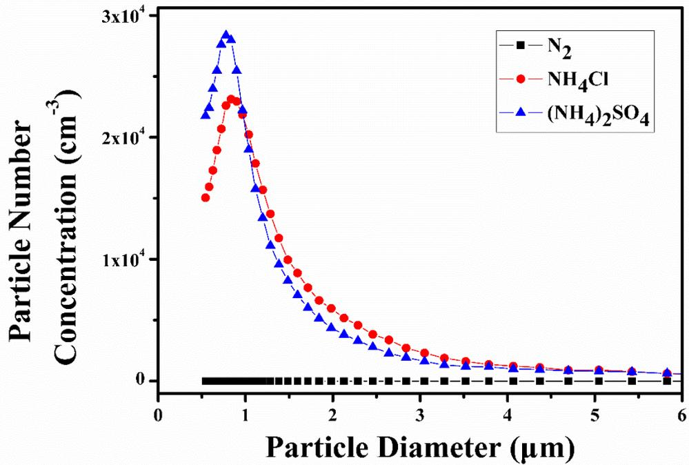
Figure S1: Size distributions of the ammonium sulfate (blue triangles) and ammonium chloride (red circles) particles we made in this work. Soon after a bag was filled with ~100L N<sub>2</sub> and ammonium aerosol particles (generated by the atomizer), the aerosols in the bag were directly detected by an Aerodynamic Particle Sizer (APS). The N<sub>2</sub> control (black squares) shows that no particles were present in the nitrogen flow used in the experiments.
