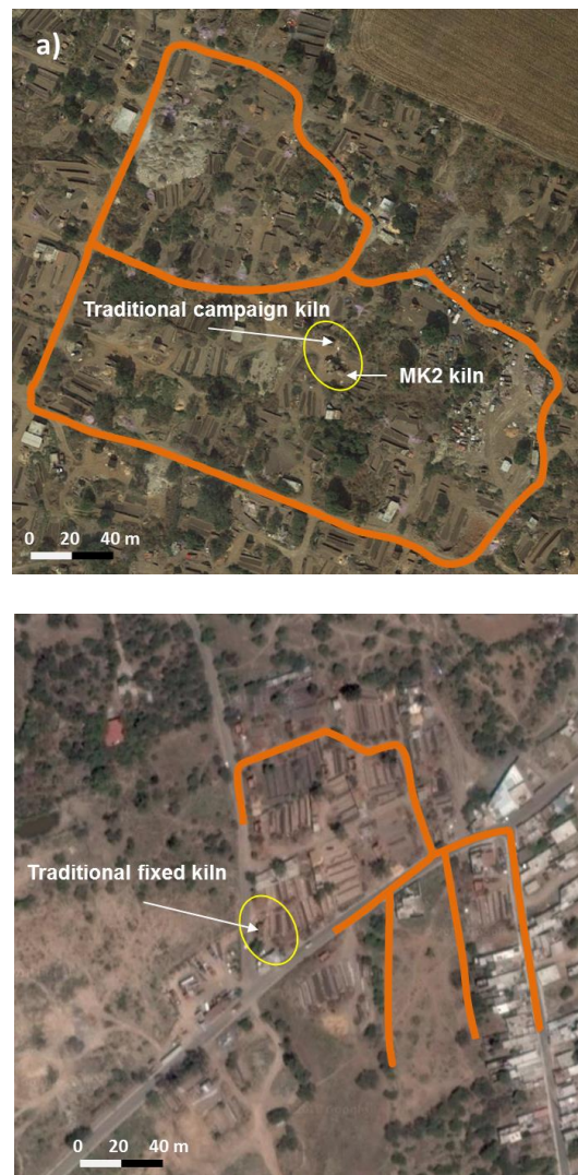
Figure S4. Locations of the sampled brick kilns: a) Traditional campaign and MK2 kilns in El Refugio, Guanajuato, Mexico, b) Traditional fixed kiln in Abasolo, Guanajuato, Mexico. Orange lines represent the sampling locations for the Aerodyne Mobile Lab using the tracer ratio sampling technique as it moved downwind the kiln depending on the prevailing wind advection patterns.
