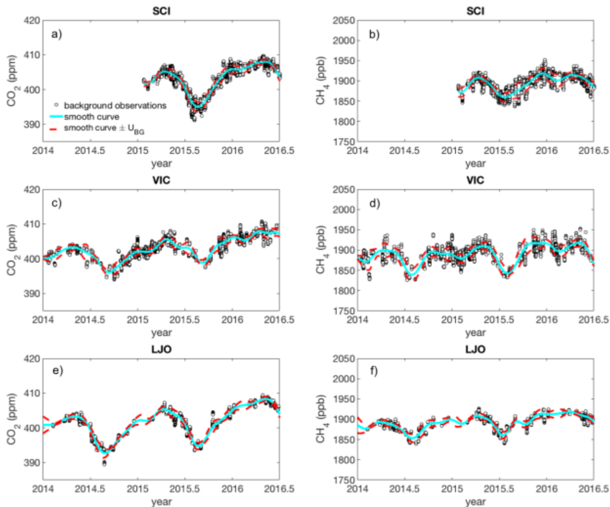
Figure S10. Background observations (black circles), smooth curve estimates (cyan lines) and uncertainty estimates (red dashed lines) for San Clemente Island (panels a-b ), La Jolla (panels c-d ), and Victorville (panels e-f ) for CO 2 and CH 4 . During 2015, the annual average uncertainty in the SCI smooth curve estimate was 1.4 ppm CO 2 and 11.9 ppb CH 4 .
