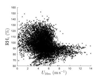
**Figure 3.** Scatter plot of observed  $RH_i$  between 60 and 160 % (from HMPmod) versus 10 m wind speed. All available half-hourly data in 2015 are plotted.
