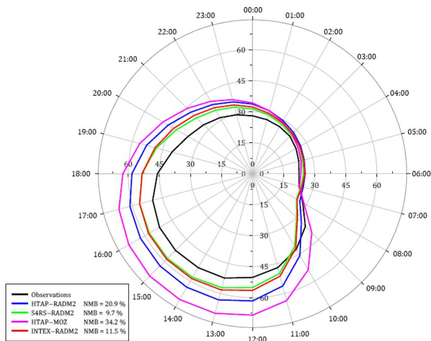
**Figure 14.** Polar plot for monthly mean diurnal variation of surface ozone (in ppbv) from all model simulations and observations, each spatially averaged over all sites. The numbers on the outermost circle represent the hour of the day, and the radial distance from the centre represents surface ozone mixing ratios in ppbv. The normalized mean biases (NMBs in %) for noontime surface ozone are indicated in the caption box.
