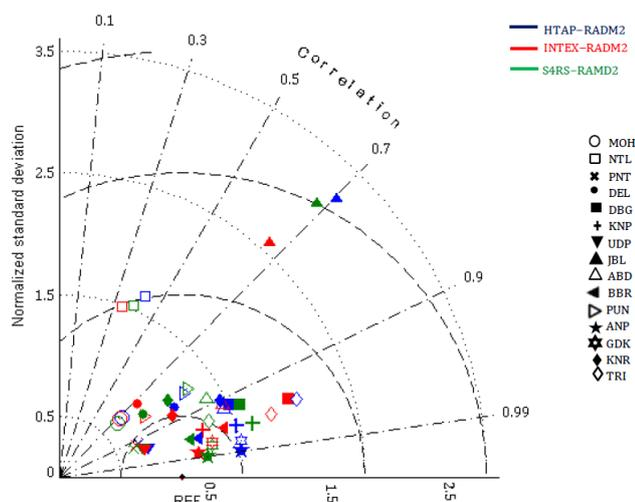
**Figure 7.** Taylor diagram with summary model statistics ( $r$ , normalized SD and RMSD) at all sites. The correlation is the cosine of the angle from the horizontal axis, the root mean square difference is the distance from the reference point (REF) and the SD is the distance from the origin.
