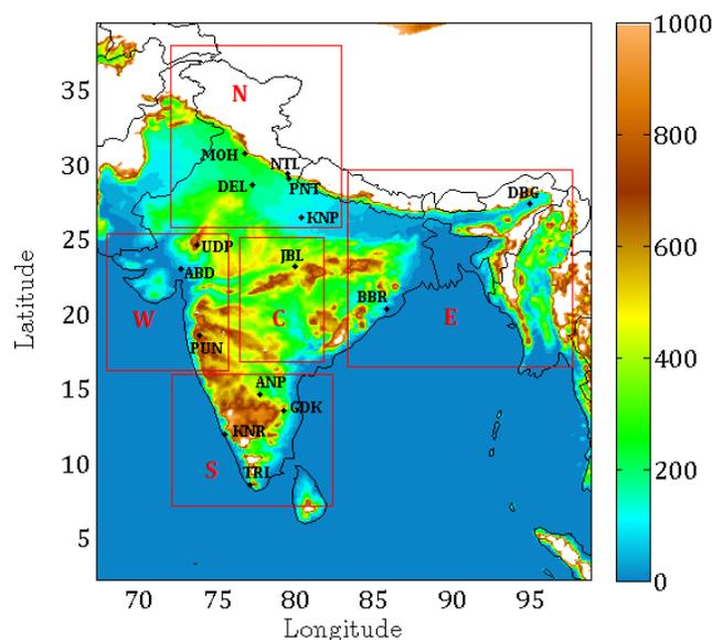
**Figure 1.** Simulation domain showing terrain height (in metres) and observation sites. The white region indicates that the terrain height is equal to or exceeds 1 km. The domain is subdivided into five regions, i.e. North (N), south (S), east (E), west (W) and central (C), as shown by red rectangles.
