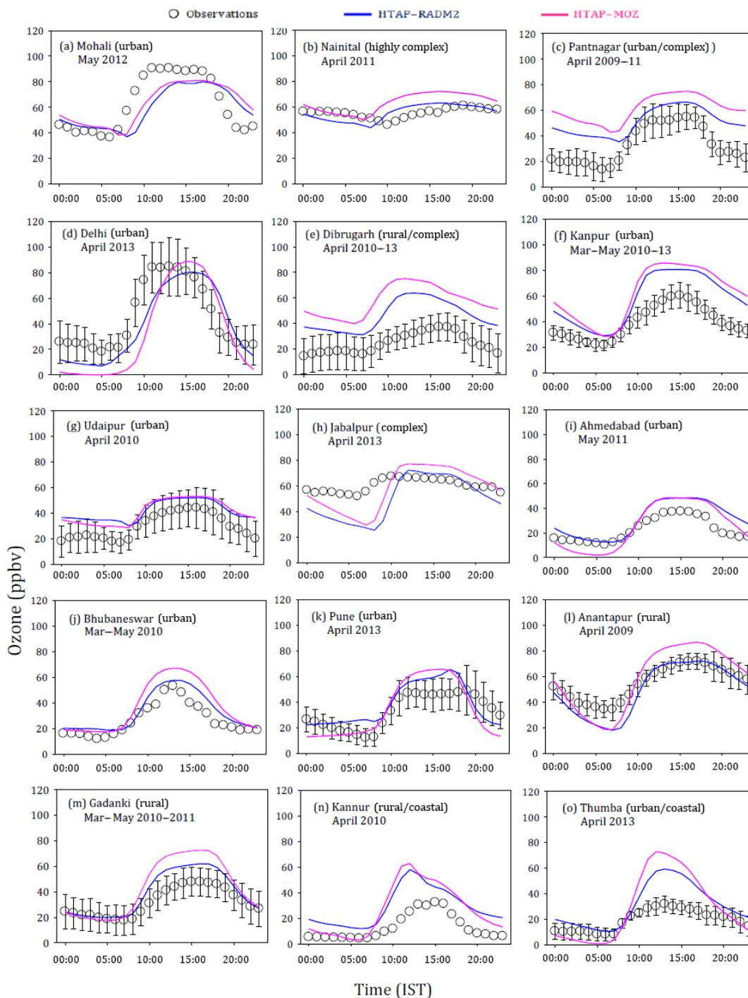
**Figure 11.** Comparison of monthly average diurnal variation of surface ozone simulated using different chemical mechanisms at various observation sites. The observational data are available for the period indicated in the figure, whereas all the model simulations are for the year 2013. Error bars represent the temporal SDs of the monthly averages. All model simulations are with the HTAP inventory.
