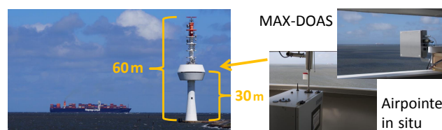
Figure 2. Radar tower Neuwerk with MAX-DOAS and the in situ measurement device.
