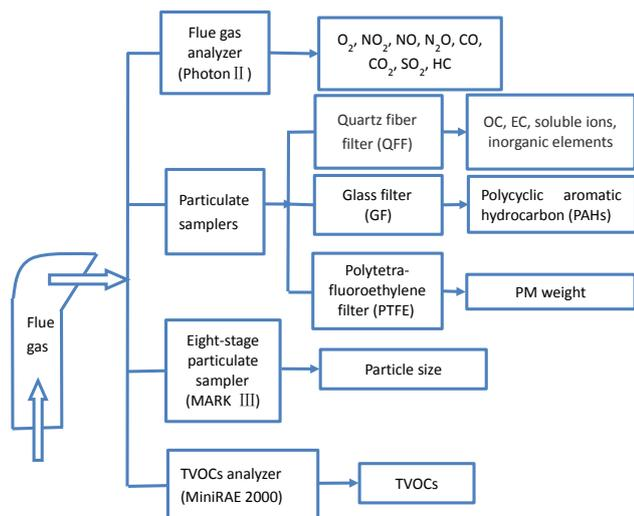
**Figure 1.** On-board emissions test system and measured analytes.
