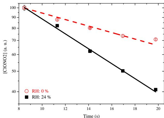
**Figure 3.** Decays of ClONO<sub>2</sub> in the flow tube due to its loss onto the Pyrex glass (circles: 0 % RH; squares: 24 % RH). Measured ClONO<sub>2</sub> mixing ratios were normalised to that at 8.5 s (when the injector was at 30 cm). Typical ClONO<sub>2</sub> mixing ratios in the flow tube are a few hundred parts per billion by volume (ppbv; see Fig. 2).
