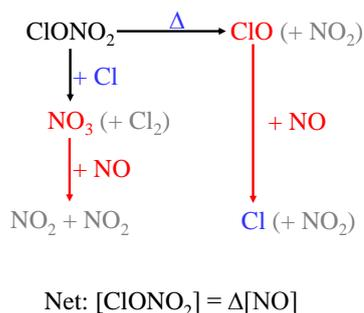
**Scheme 1.** The ClONO<sub>2</sub> detection scheme used in our work.
