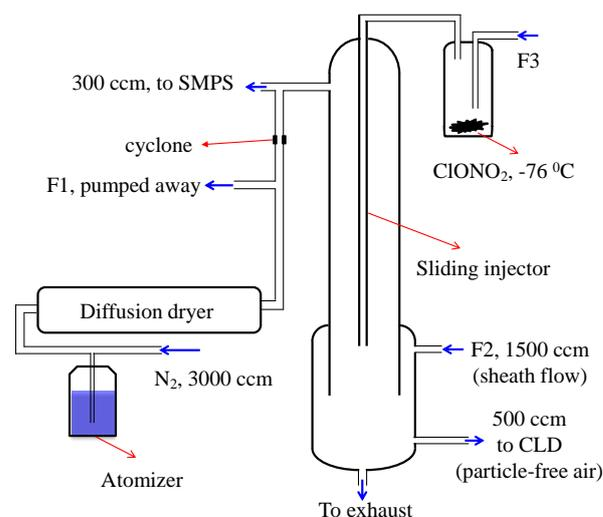
**Figure 1.** Schematic diagram of the aerosol flow tube used in this study. SMPS: scanning mobility particle sizer; CLD: chemiluminescence detector, used to measure the ClONO<sub>2</sub> concentration (measured as the change in NO concentration). All the flows (except the flow applied to the atomiser) were controlled by mass flow controllers. Flow details are provided in the text.
