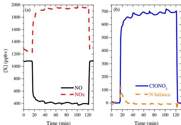
**Figure 2.** Response of measured NO and NO<sub>x</sub> mixing ratios to the introduction of ClONO<sub>2</sub> into the flow tube (left panel). The corresponding calculated ClONO<sub>2</sub> mixing ratio and nitrogen balance are also shown (right panel).
