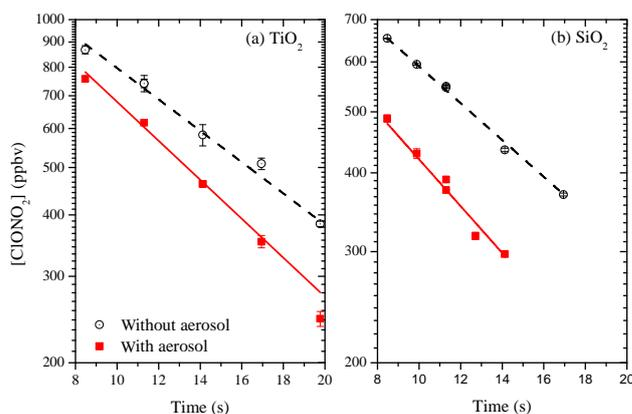
**Figure 4.** Decays of ClONO<sub>2</sub> in the aerosol flow tube without (open circles) and with (solid squares) aerosol particles in the aerosol flow tube under different experimental conditions. **(a)** TiO<sub>2</sub> with a surface area concentration of  $2.3 \times 10^{-3} \text{ cm}^2 \text{ cm}^{-3}$  at 33 % RH; **(b)** SiO<sub>2</sub> with a surface area concentration of  $2.9 \times 10^{-3} \text{ cm}^2 \text{ cm}^{-3}$  at 39 % RH.
