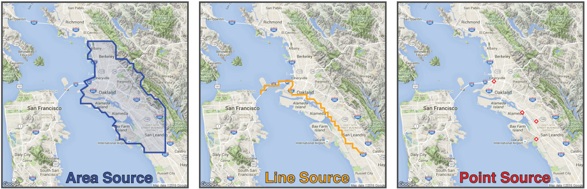
Figure 5: Source types examined. Same as right column from main text Fig. 4. The area source, line source, and point source have emission rates of 147 \pm 55 tC hr -1 , 45 \pm 20 tC hr -1 , and 9 \pm 4 tC hr -1 over one week, respectively.
