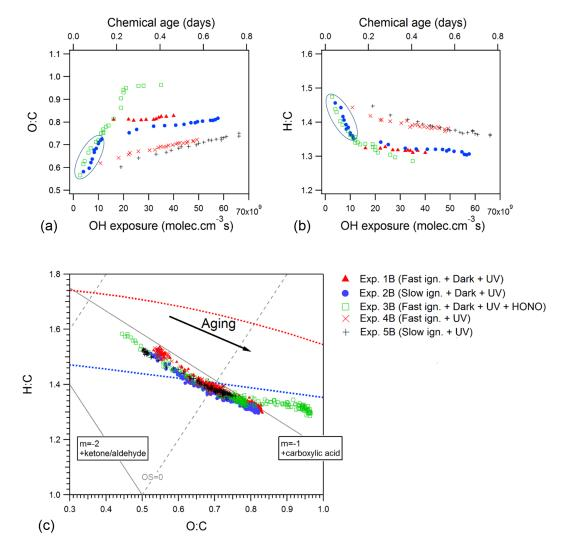
**Figure 4.** Comparison of OA elemental composition for the second set of experiments (Exp. 1B–5B): OA elemental composition vs. OH exposure (**a–b**) and van Krevelen diagram (**c**). The improved-ambient method from Canagaratna et al. (2015) was applied for the elemental analysis. The dotted lines define the triangular space where ambient OA components are typically located (Ng et al., 2010) and dark aging periods are circled in grey (**a–b**).
