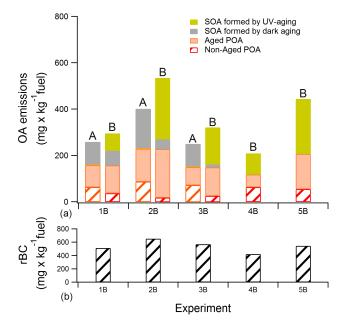
**Figure 6.** Aged and non-aged POA emission together with SOA at the end of dark (**a**) and UV aging (**b**) periods based on PMF calculations (Exp. 1B-5B) as well as (**b**) refractory black carbon (rBC) emissions.
