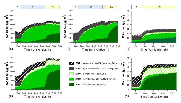
**Figure 5.** Evolution of OA during aging based on PMF calculations: (a) Exp. 1B (fast ignition), (b) Exp. 3B (fast ignition), (c) Exp. 4B (fast ignition), (d) Exp. 2B (slow ignition) and (e) Exp. 5B (slow ignition). The stabilization phase is marked as S, dark aging as D, the HONO addition as H and UV aging as UV in the upper panel.
