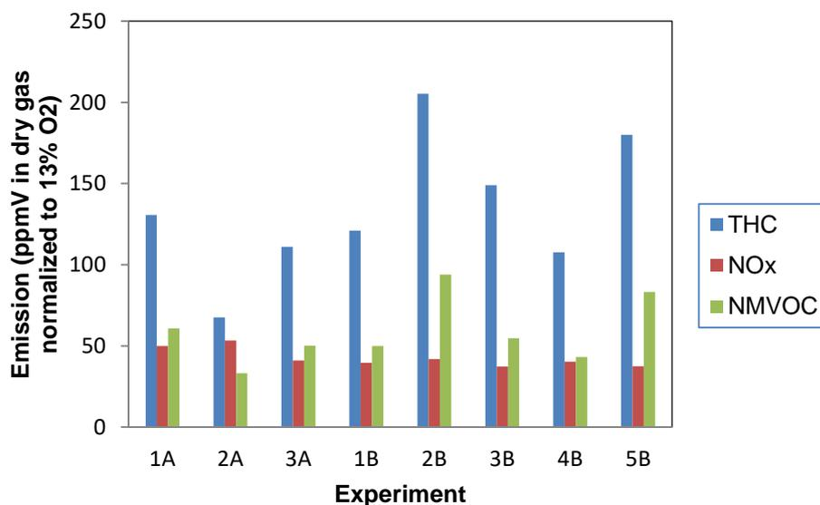
Figure S1: Total hydrocarbon (THC), NO<sub>x</sub> and non-methane VOC (NMVOC) emissions (FTIR) from logwood emissions for all experiments.
