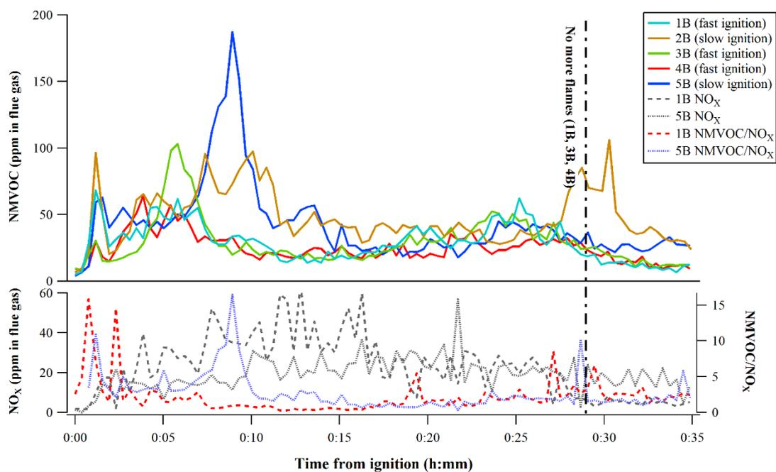
Figure S3. Time series from emissions of non-methane VOC and nitrogen oxides and their ratio. Measured with FTIR from raw flue gas. Dash line indicates a point at fast ignition experiments when visible flames extinguished and only char burning continued.
