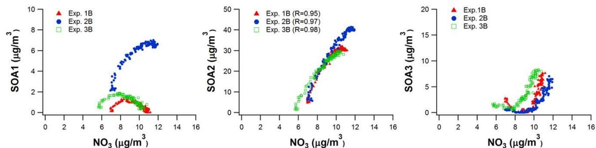
Figure S7: PMF factors (a) SOA1, (b) SOA2 and (c) SOA3 vs. particulate nitrate during dark aging and corresponding correlation coefficients (R) for SOA2.
