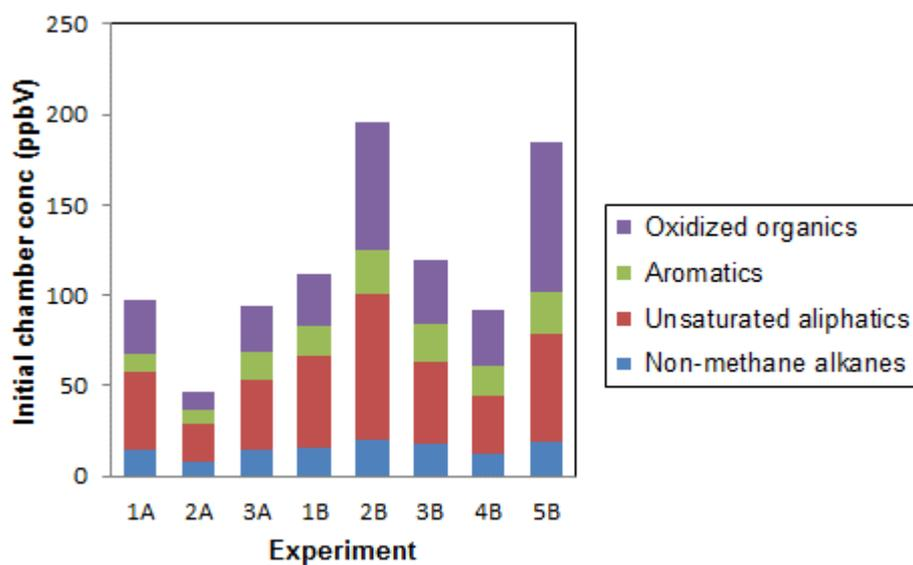
Figure S2: Gas-phase organic emissions (FTIR) from logwood combustion for all experiments. Emissions are calculated for initial chamber concentrations.
