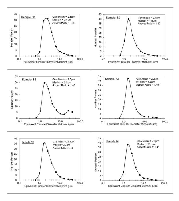
**S01**. Particle size distributions, as well as size and shape statistics for  $<38 \mu m$  sieved samples S1–S6, as measured by scanning electron microscopy (SEM).
