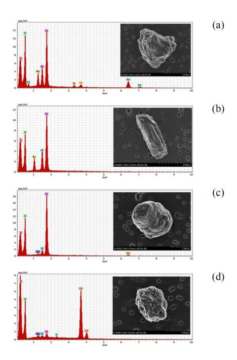
**S03**. Secondary electron images and energy dispersive spectra (EDS) of soil particles (**a**) sample S5, Fe bearing clay mineral possibly illite. (**b**) sample S8, albite feldspar crystal. (**c**) sample S11, rounded quartz grain with minor amount of clay. (**d**) sample S11, cluster of calcite crystals with small amounts of clay and gypsum.
