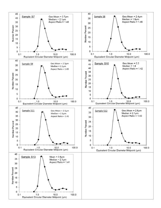
**S02**. Particle size distributions, as well as size and shape statistics for <38 μm sieved samples S7–S13, as measured by scanning electron microscopy (SEM).
