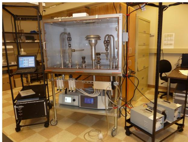
**Figure 2.** Integrated dust entrainment facility: three-wavelength photoacoustic instrument (DMT PASS-3) on rack to the left, re-suspension chamber on trolley in the center, with a particle size analyzer and beta-attenuation gauge installed below the chamber, and an array of vacuum pumps on rack to the right.
