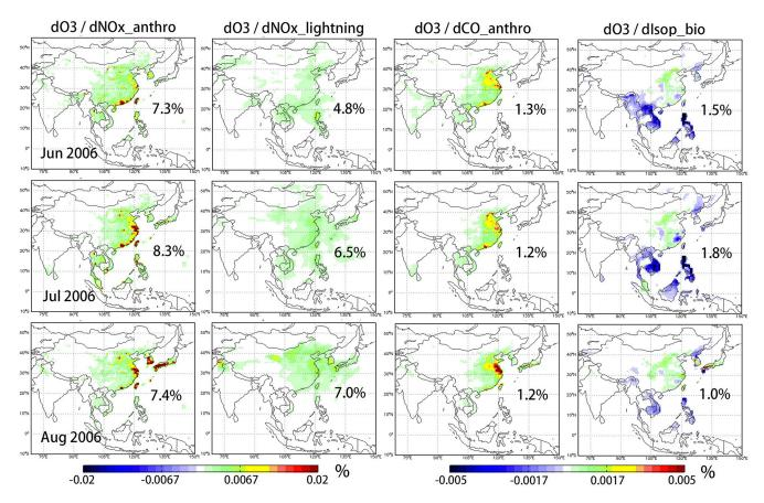
Figure 6. Contributions of anthropogenic  $NO_x$ , lightning  $NO_x$ , anthropogenic CO, and biogenic isoprene on free tropospheric (819–396 hPa)  $O_3$  over China outflow region derived from the adjoint of GEOS-Chem in June, July and August 2006.
