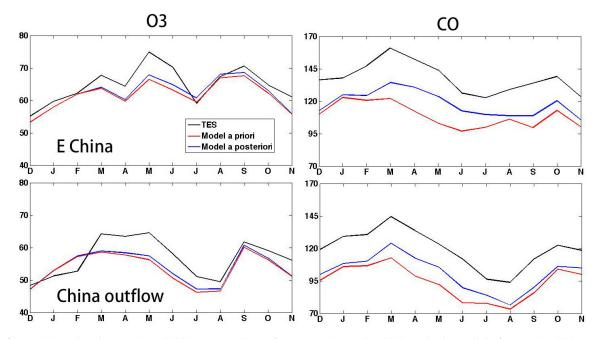
**Figure 4.** Monthly regional mean  $O_3$  and CO concentration at free troposphere (681–383 hPa) in the period of December 2005–November 2006. The red line is GEOS-Chem model simulation with a priori emission inventories. The blue line is model simulation with updated  $NO_x$  and CO emission inventories. The black line represents TES measurements. The model results are smoothed with the TES averaging kernels. The positive bias in the TES  $O_3$  data is larger in summer and smaller in winter.
