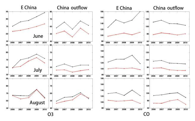
**Figure 2.** Monthly regional mean  $O_3$  and CO concentration at free troposphere (681–383 hPa) in June, July and August 2006–2010. The red line is the GEOS-Chem model simulation with a priori emission inventories and the black line represents the TES measurements. The model results are smoothed with the TES averaging kernels. The TES ozone data are biased high by 7 ppbv.
