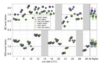
Figure 7. BC (top panel) and  $NO_x$  (bottom panel) emission error factors (EEFs) for each individual flight (when available) and averaged EEF (on the right) at the 95 % confidence interval, for all six simulated cases (logarithmic scale).
