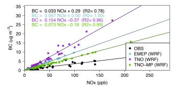
**Figure 4.** Observed and simulated BC vs.  $NO_x$  concentrations at LHVP between 05:00 and 08:00 UTC considering July flight days, and linear fits (lines). Only simulations with WRF meteorological data are reported here.
