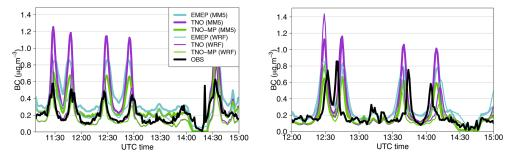
Figure 6. Observed (in black) and simulated BC concentrations along the aircraft trajectory for 10 (left panel) and 13 July (right panel).
