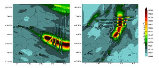
**Figure 5.** Observed (along the aircraft trajectory) and modeled (in the background, with the TNO-MM5 case) BC concentration for 10 (left panel) and 13 July (right panel). Paris and some other large cities are indicated. Simulated concentrations shown here are taken at 13:00 UTC on the fourth layer, which roughly corresponds to 470–870 m height. The solid black line corresponds to the flight path outside that layer (altitude above 870 or below 470 m).
