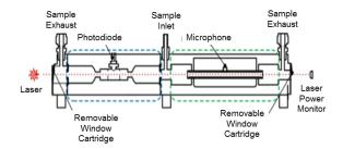
**Figure 2.** Diagram showing the scattering (blue dashed region) and absorption (green dashed region) cells in the Photoacoustic Extinctiometer (PAX).
