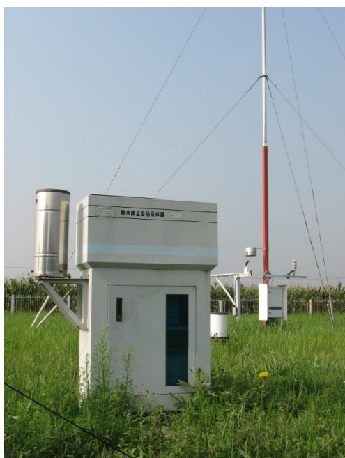
Figure S1. The automated wet and dry deposition sampler used in this study. The agricultural station of Yucheng in Shandong Province (left) and a schematic diagram of the sampler with the main apparatus (right): rainfall sampler (a), dry deposition bucket (b), and PUF filter for sampling dry deposited particles (c).
