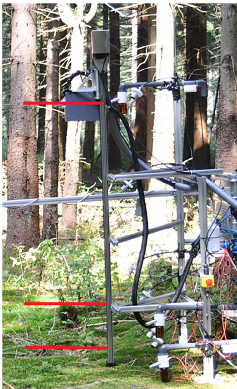
Figure S2: External sampling unit of the LOPAP (grey box) and inlet for NO x installed on the lift system at the forest floor. Three positions (1.6 m, 0.4 m and 0.1 m) used for the profile measurements are indicated in red.
