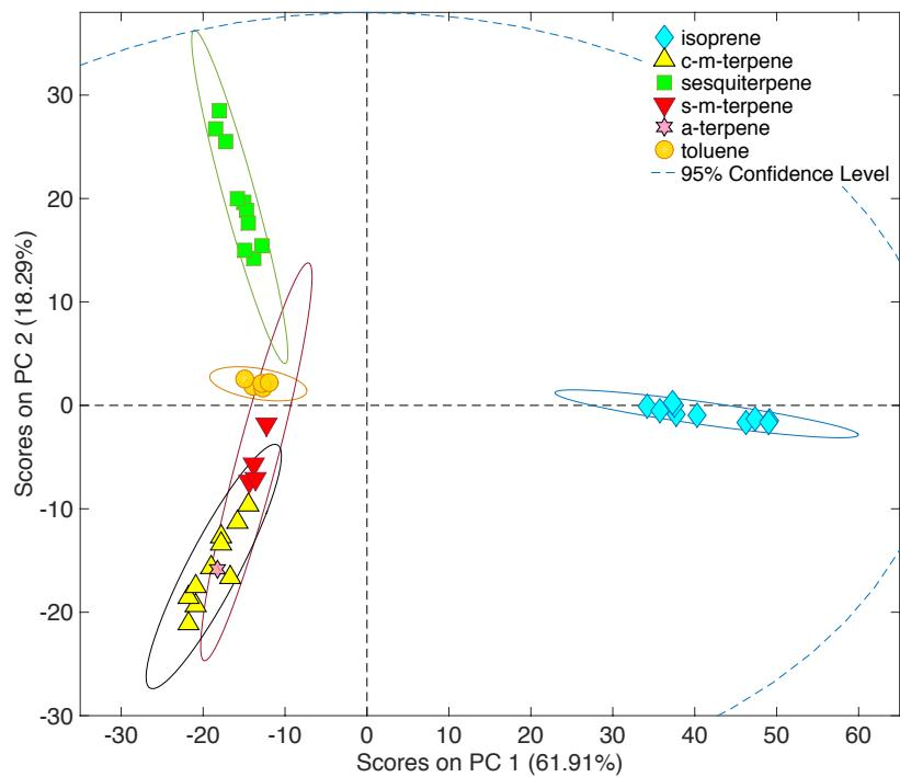
Figure S1: PCA scores plot of the second vs. first principal components derived from the PCA analysis of the toluene test set using the PCA model developed from the isoprene, cyclic monoterpene ( $\alpha$ -pinene and limonene), sesquiterpene ( $\beta$ -caryophyllene), straight chain monoterpene (myrcene and linalool) and  $\alpha$ -terpinene chamber data. Classification confidence levels = 95 %.
