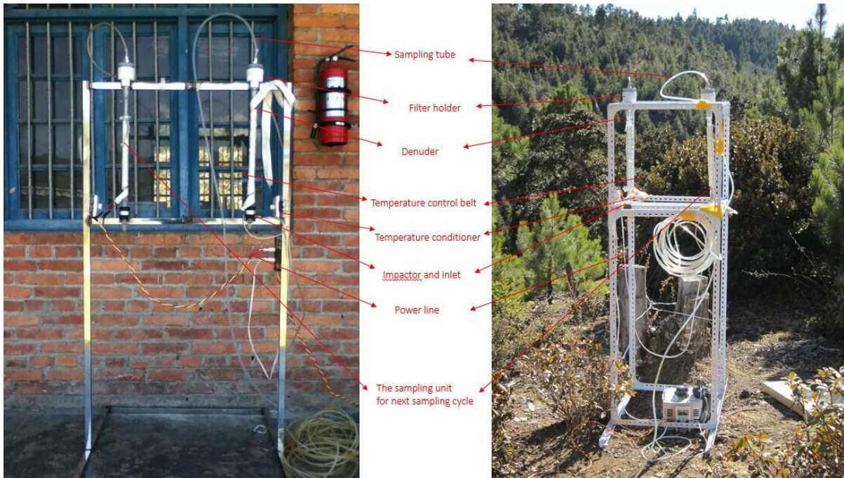
Fig.S3: The picture of denuder-based sampling unit.
