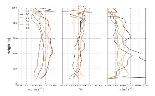
**Figure 7.** Profiles of the standard deviation ( $\sigma_w$ ) and skewness ( $\gamma_w$  of vertical velocity and the dissipation rate ( $\epsilon$ ) for 1 h segments during the early hours of 25 February.
