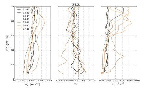
**Figure 6.** Profiles of the standard deviation ( $\sigma_w$ ) and skewness ( $\gamma_w$ ) of vertical velocity and the dissipation rate ( $\epsilon$ ) for 1 h segments during the early hours of 24 February.
