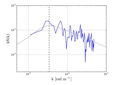
**Figure 1.** An example of a vertical velocity power spectral density (*S*) as a function of the wave number *k* (blue line) taken from roughly the middle of the well-mixed layer on 25 February at 04:00 UTC. The thin grey line represents the fit from Eq. (3). The black dashed line shows the wave number corresponding to  $\lambda_0$  in this particular example. The inertial subrange is found for wave numbers above this point.
