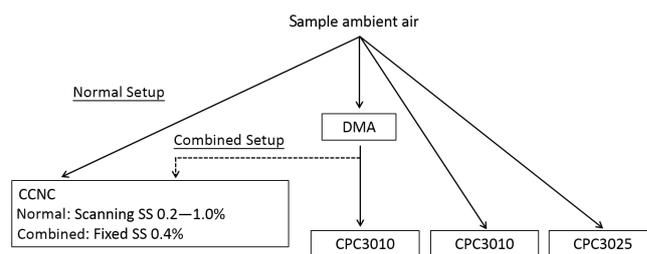
**Figure 1.** Scheme of the two different measurement modes for the cloud condensation nuclei counter (CCNC). When CCN size-resolved number concentration measurements took place, the CCNC was connected behind the Differential Mobility Analyzer and the supersaturation was set to 0.4 %. During normal operation, the CCNC was connected parallel to the DMA and SS alternated between 0.2 and 1.0 %.
