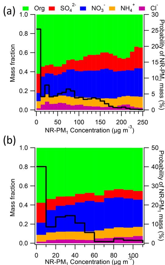
**Figure 5.** Submicron aerosol composition as a function of NR-PM<sub>1</sub> mass loadings (a) before APEC and (b) during APEC. The solid line shows the probability of NR-PM<sub>1</sub> mass.
