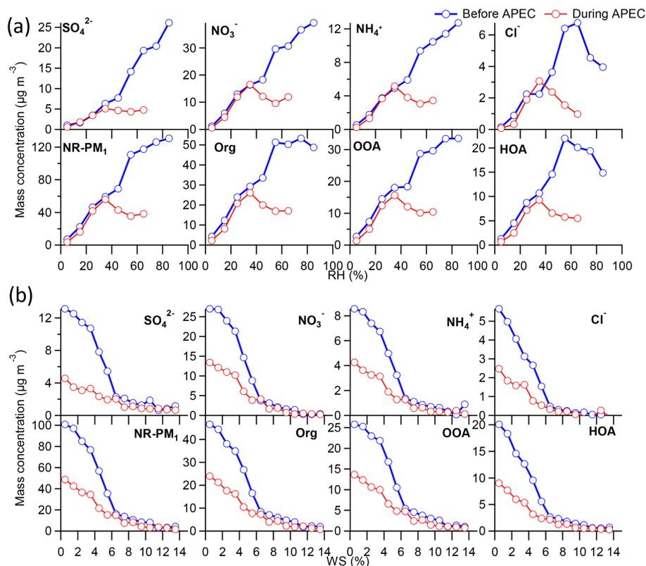
**Figure 8.** Variations of NR-PM<sub>1</sub> species and OA factors as a function of (a) RH and (b) WS before and during APEC. The RH and WS were from the tower measurements at 280 m.
