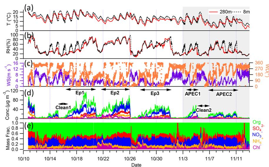
**Figure 2.** Time series of (a)  $T$ , (b) RH, (c) WS and WD, and (d) concentrations of NR-PM<sub>1</sub> species (Org, SO<sub>4</sub><sup>2-</sup>, NO<sub>3</sub><sup>-</sup>, NH<sub>4</sub><sup>+</sup>, and Cl<sup>-</sup>), and (e) mass fraction of each species in NR-PM<sub>1</sub>. Two clean periods and five haze episodes are marked in (d) for further discussions. The meteorological parameters in this figure were all from the tower measurements.
