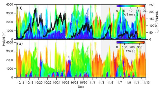
**Figure 1.** Evolution of vertical profiles of (a) wind speed (WS) and (b) wind direction (WD) from the measurements of the Doppler wind lidar. The time series of NR-PM<sub>1</sub> (i.e., Org + SO<sub>4</sub><sup>2-</sup> + NO<sub>3</sub><sup>-</sup> + NH<sub>4</sub><sup>+</sup> + Cl<sup>-</sup>) is shown as the black line in (a). The shaded area refers to the APEC period (same for following figures).
