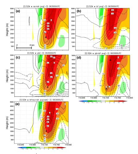
**Figure 16.** As in Fig. 14, except for  $w (m s^{-1}, \text{ color, scale at bottom)}$  and the vertical (z) component of perturbation pressure gradient force  $(10^{-3} m s^{-2}, \text{ contours, every } 15 \times 10^{-3} m s^{-2}, \text{ dashed for negative values)}$  from (a)  $p'_d$ , (b)  $p'_b$ , (c) buoyancy (B), (d)  $p'_b + B$ , and (e)  $p'_d + p'_b + B$ , respectively. The positive and negative centers are labeled by plus and minus signs, respectively.
