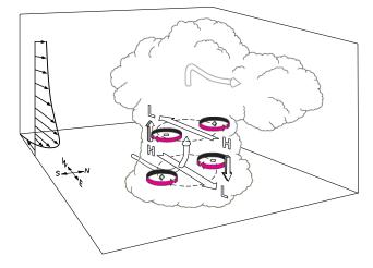
**Figure 6.** A schematic showing the distribution of dynamical pressure perturbations (marked by "H" for anomalous high and "L" for anomalous low) relative to a mature storm cell in an environment with the presence of a westerly low-level jet (LLJ) and westerly (easterly) vertical shear below (above) the jet core as in our case. The configuration is in favor of new development at the rear side and a slower moving speed of the cell.
