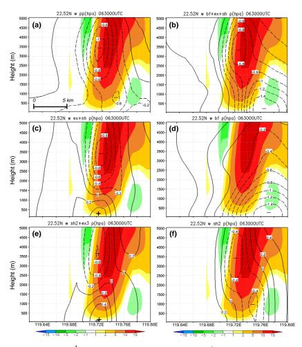
**Figure 15.** As in Fig. 14, except for w (m s<sup>-1</sup>, color, scale at bottom) and (a) total p' (hPa, contours, every 0.2 hPa, dashed for negative values) separated from the background, and (b)  $p'_b + p'_d$ , (c)  $p'_d$ , (d)  $p'_b$ , (e) the portion of  $p'_d$  from SH2 and EX3, and (f) the portion of  $p'_d$  from SH2 alone (all in hPa, contours) in Eq. (13) solved by the relaxation method. The positive and negative centers are labeled by plus and minus signs, respectively.
