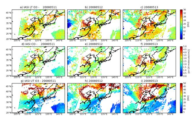
Figure 5. Panels (a–c): lower-tropospheric ozone columns (surface to 6 km a.s.l) retrieved from IASI from 11 to 13 May 2008. Panels (d–f): total CO columns retrieved from IASI. Panels (g–i): upper-tropospheric ozone columns (6 to 12 km a.s.l.) retrieved from IASI.
