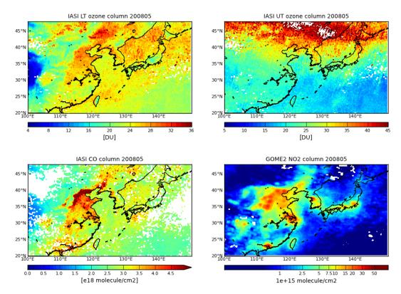
Figure 9. Monthly lower (upper left) and upper (upper right) tropospheric ozone columns observed by IASI in May 2008 as well as monthly IASI total CO columns (lower left) and GOME-2  $NO_2$  tropospheric columns (lower right) observed in May 2008. The average is calculated for a  $0.25^{\circ} \times 0.25^{\circ}$  resolution grid.
