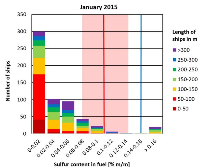
**Figure 4.** Detailed view of the January 2015 data set. The lengths of the ships are colour-coded; the red line indicates the 0.1 % limit, with the shaded area representing the upper limit uncertainty of 30 %. The blue line indicates the suggested limit of 0.15 % for flagging ships as exceeding the sulfur fuel content limit allowed.
