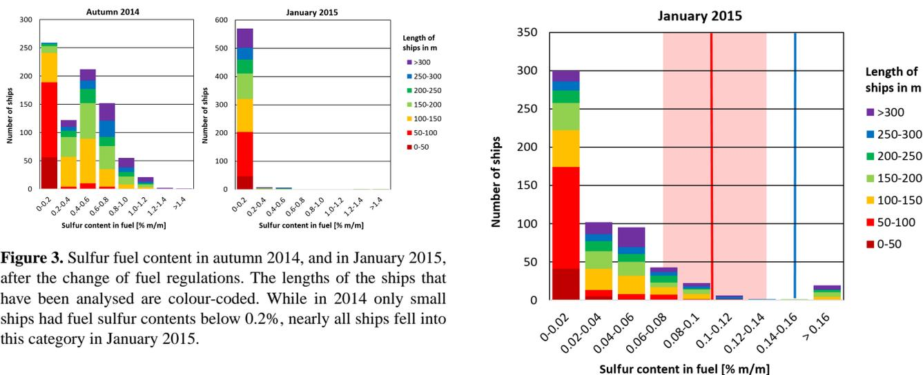
**Figure 3.** Sulfur fuel content in autumn 2014, and in January 2015, after the change of fuel regulations. The lengths of the ships that have been analysed are colour-coded. While in 2014 only small ships had fuel sulfur contents below 0.2%, nearly all ships fell into this category in January 2015.
