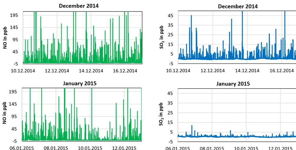
**Figure 2.** Comparison of absolute NO and SO<sub>2</sub> volume mixing ratio values measured over 2 weeks, 1 week in December 2014 and 1 week in January 2015 with comparable wind conditions. Each peak belongs to one emission plume of an individual ship. The reduction in SO<sub>2</sub> in 2015 is obvious, while for NO, no reduction can be observed.
