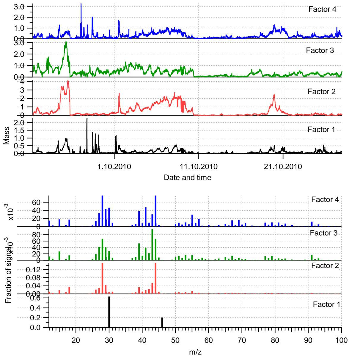
**Figure S3.** Time series and mass profiles by PMF analysis at four-factor solution with  $f_{\text{Peak}} = +0.1$ .
