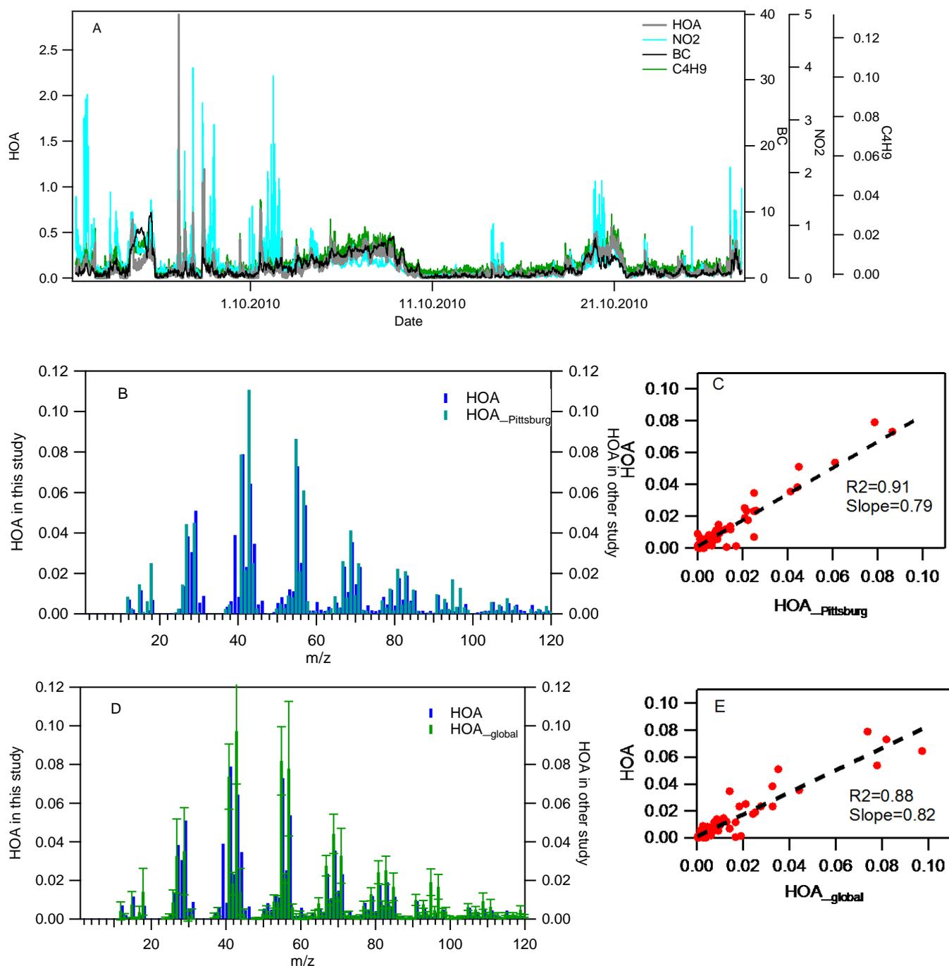
**Figure S9.** (A) Correlations of HOA time series with tracers; (B) Comparison of HOA mass spectrum from HOA determined in Pittsburg (Ulbrich et al., 2009); (C) a scatter plot of HOA mass spectrum between this study and Pittsburg; (D) Comparison of HOA mass spectrum from HOA determined on a global scale (Ng et al., 2010); (E) a scatter plot of HOA mass spectrum between this study and on a global scale;
