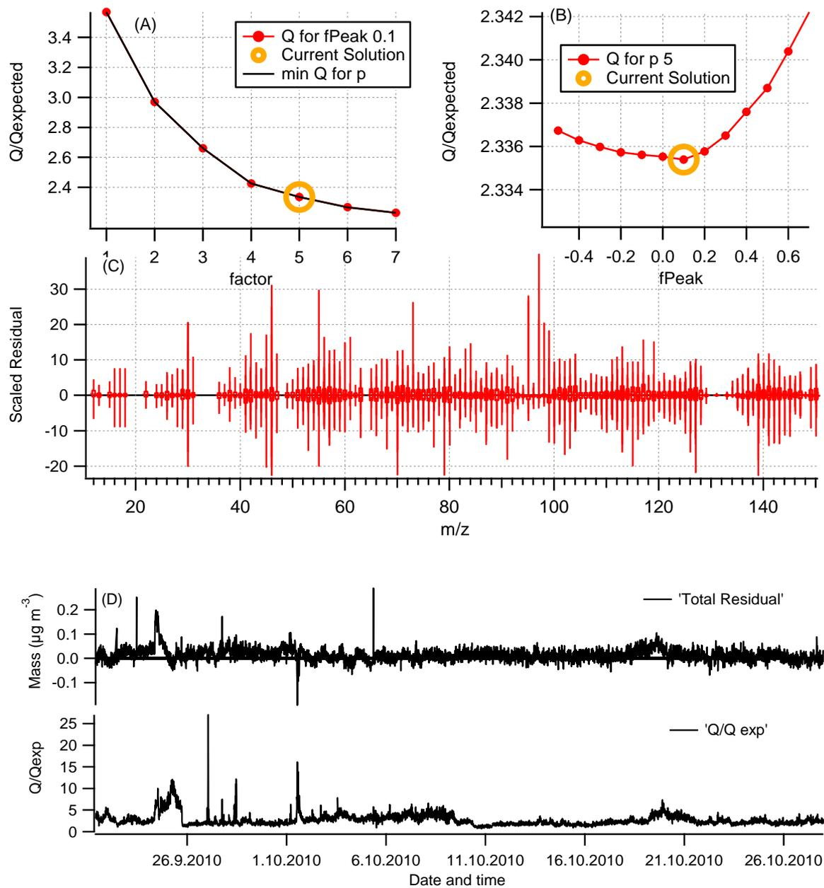
**Figure S1** PMF key diagnostics plots: (A)  $Q/Q_{\text{expected}}$  varies as function of PMF factor at  $f_{\text{Peak}} 0.1$ ; (B)  $Q/Q_{\text{expected}}$  varies as function of rotational ambiguity; (C) Scaled residual for each mass; (D) time series of the total residual and  $Q/Q_{\text{exp}}$  contribution for every point during this study. For more details on PMF and the interpretation of these plots see Ulbrich et al. (2009).
