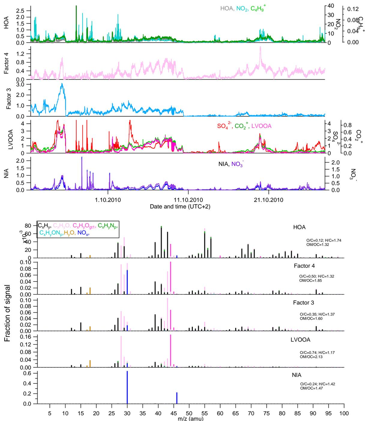
**Figure S2.** Time series and mass profiles by PMF analysis at five-factor solution. Factor 3 and 4 were merged to generate a new factor by a mass-weighted combination, which results are reported in the paper. HOA, hydrocarbon-like organic aerosol; LVOOA, low-volatile oxygenated OA; NIA, nitrate inorganic aerosol
