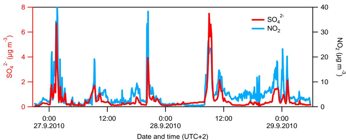
**Figure S7.** Comparisons of time series of  $\text{SO}_4^{2-}$  and  $\text{NO}_2$  during the primary aerosol emitting days, which is shown in the gray bar in Figure 1. Good correlation of  $\text{SO}_4^{2-}$  with  $\text{NO}_2$  suggests that the  $\text{SO}_4^{2-}$  is primary in nature during this period.
