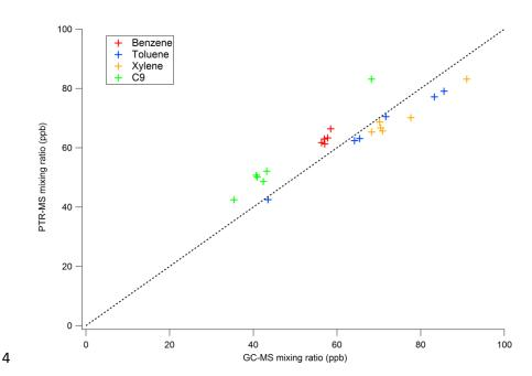
5 Figure S3. A comparison between PTR-MS and GC-MS for C<sub>6</sub>-C<sub>9</sub> aromatics measured in the
