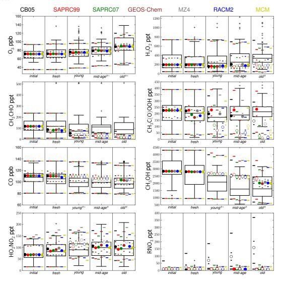
Fig. 5. Simulation results (circle: median; bars: 0, 25, 75, 100 percentiles) and observations (box and whisker) binned by  $NO_X$ :HNO<sub>3</sub>. For observations, each age category is superscripted for statistical difference (p < 0.0001) from the preceding (\*) and fresh (#) age group. For model predictions, the median for each chemical mechanism is left hollow when statistically different (p < 0.0001) from the observations.
