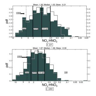
**Fig. A4.** Observed  $NO_x$ :HNO<sub>3</sub> (bars; left: CIT, right: UNH) compared to simulated (lines) from the GEOS-Chem chemical mechanism using the optimized, bias-corrected statistical model.
