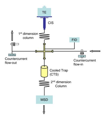
**Figure S1.** Schematic diagram of the 2-dimensional GC-MS system. Figure also appears in Ma and Hays, 2008.
